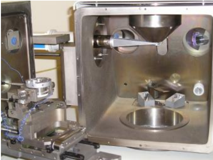
Centaurus Detector in use on Leo SEM chamber
